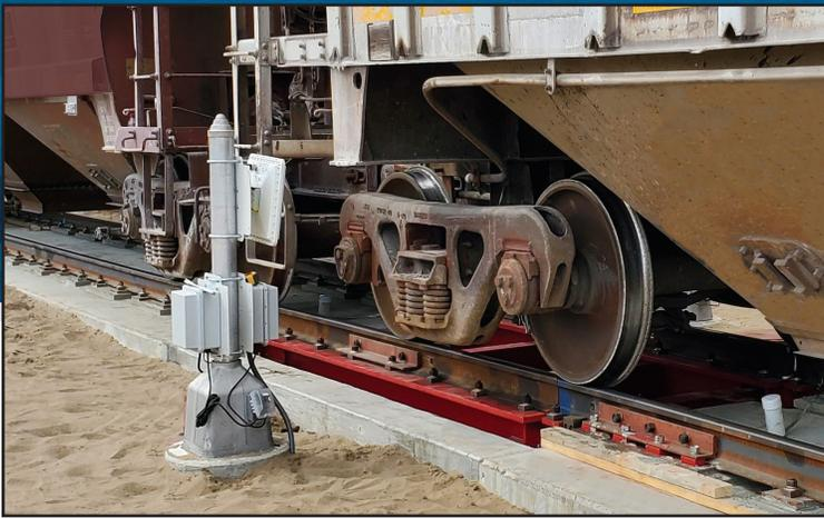
The weigh-in-motion system includes two heavy-duty aluminum pole kits which are installed adjacent to the rail line, on either side of the scale. Each pole is used to position a TransCore® RFID railroad car tag reader (top of pole facing train) and support two secure aluminum cabinets that store the power supply and communication components for the attached tag reader and system wheel sensors.
